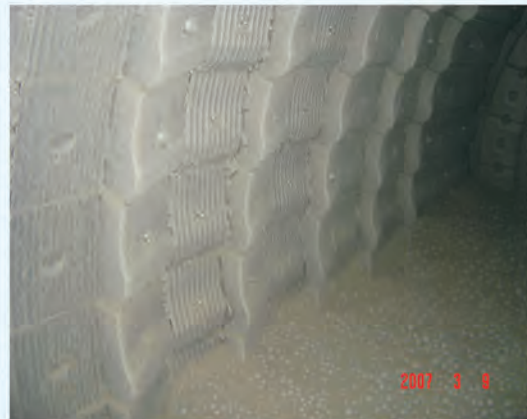
Φ3.8×13m水泥磨沟槽衬板与锥面衬板组合 Combined grooved liners in 2nd chamber Φ3.8×13m
